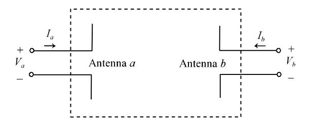
The source integrals in the general 3-D reciprocity theorem of Equation (8) simplify to line integrals for the case of wire antennas.
